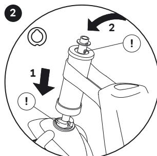
Remove transport restraint (paperboard, rubber band) and take off the washer.
