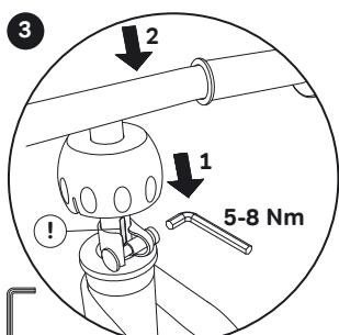
Slide the handlebar all the way onto the fork shaft, and tighten the screw. Align the slot in the handlebar with the rear (!) Firmly press down on the spherical cap until it snaps into position.
